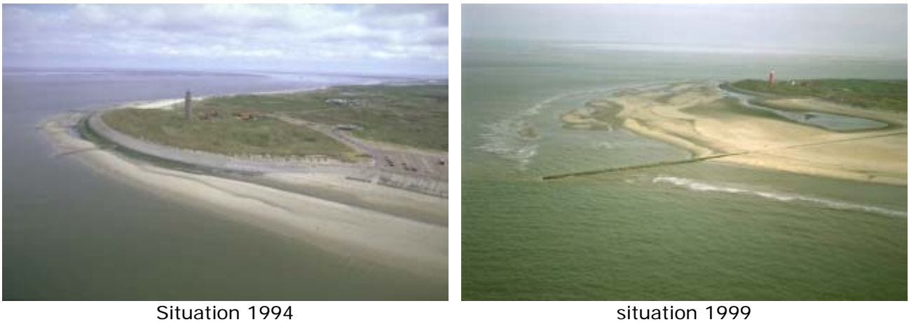
Fig. 12: Effect cross-shore dam at island Texel.
